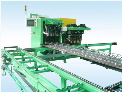
상/하현재 Welding Unit 1 [Inlet]
