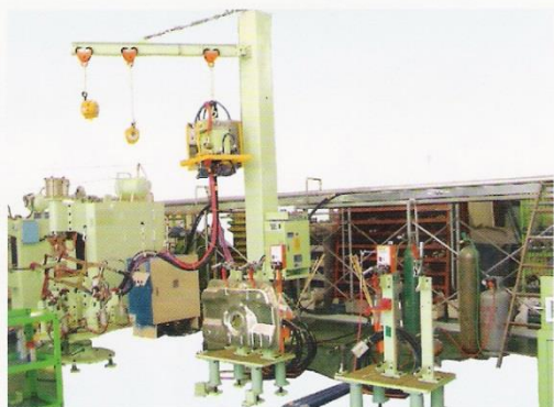
B/K, RING SPOT WELDING LINE
