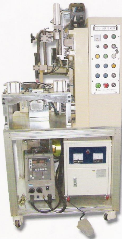
SHELL / LINER TIG WELDING M/C
